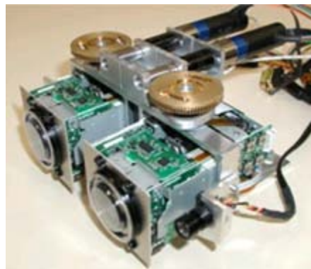
Figure 2. Robonaut Robotic Vision Platform
